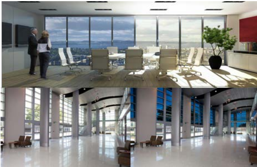
Figure 6: Before and after examples of Electrochromic Smart Glass in use
